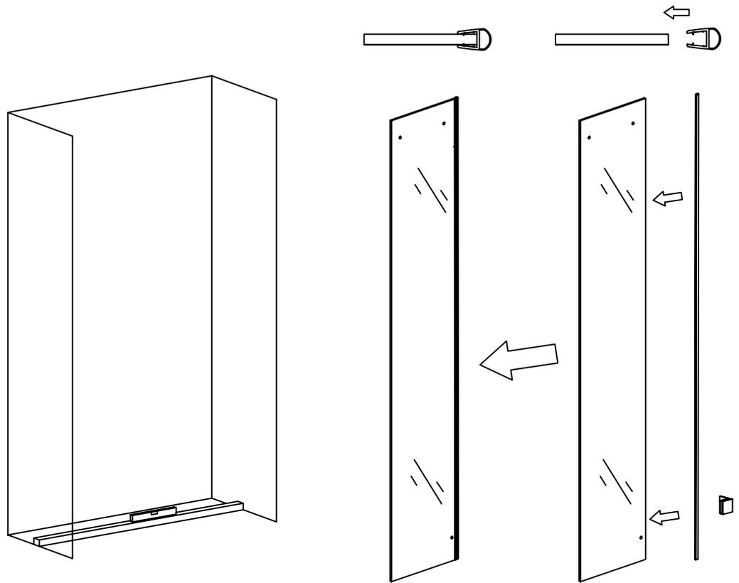
1. Select the installation position, put the base stone or tray to the position and measure it vertically by spirit level.
