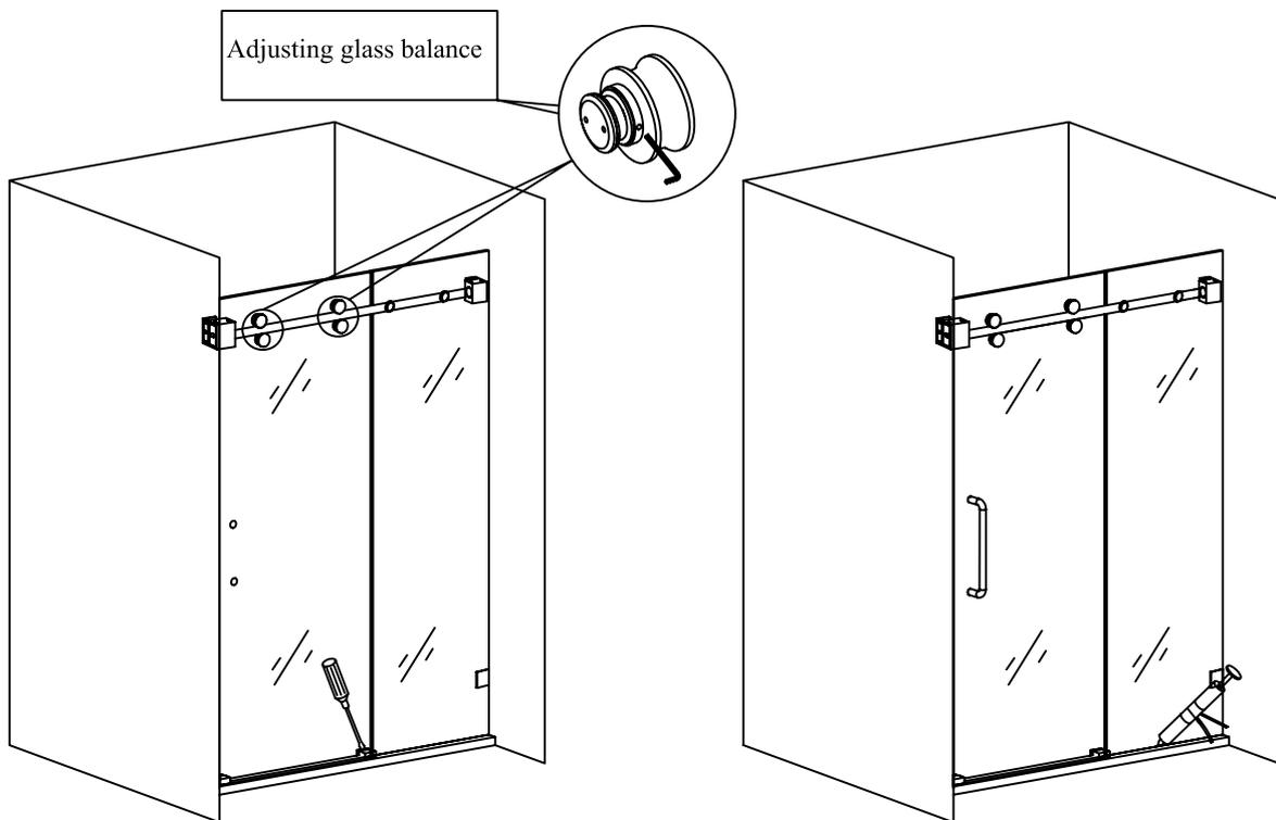
1. Put the waterproof bar on the base stone, locked it tight with tapping screw.
