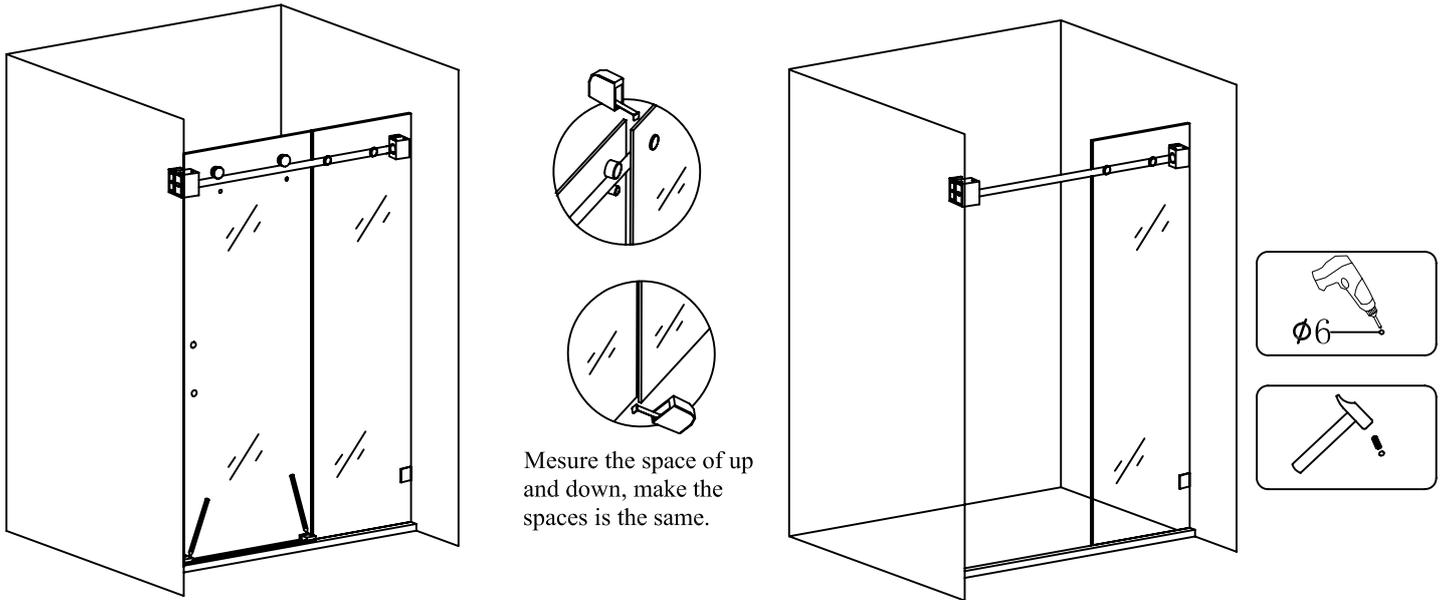
1. Put two plastic sliding cover and movable glass onto the base stone. Measure the space between the movable glass and fixing glass, make them vertically. Mark the sliding cover position by pencil, take off movable glass and sliding cover, then drill a hole by a Ø6 driller and insert with inflatable rubber.
