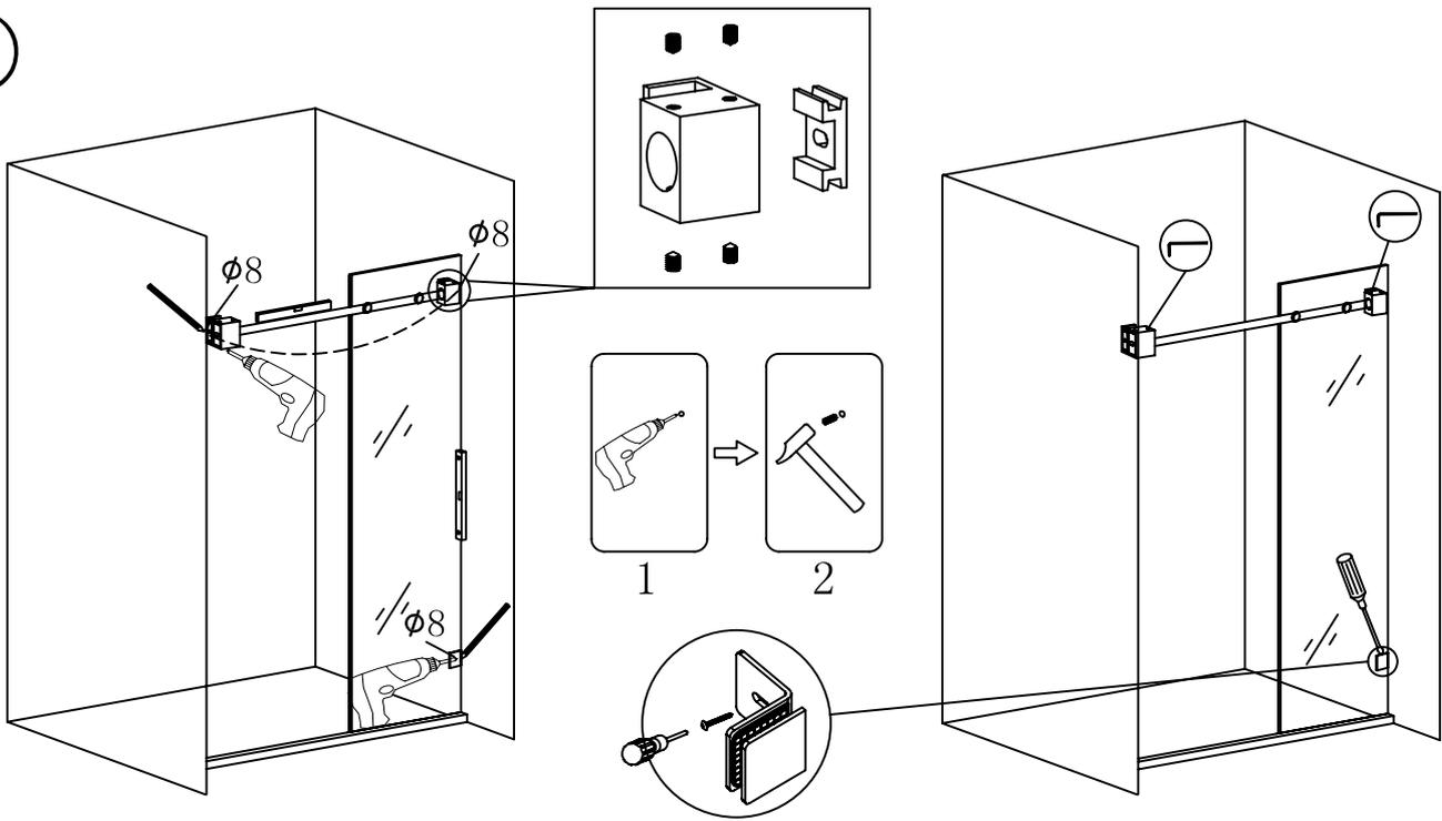
1. Put the fixing glass on the base stone, measure and make the upper rail and fixing glass vertically by spirit level, marked by pencil, then take off the fixing glass.
